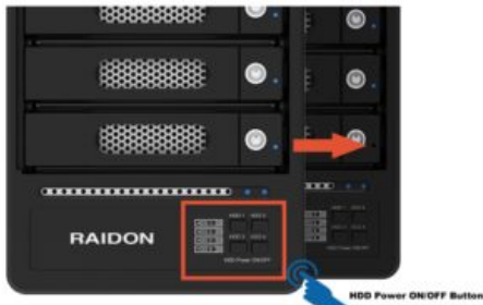
4 hard drive independent power switches
