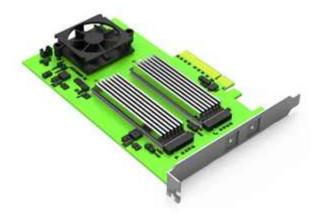
The HPD08-2 HBA boasts fast data transfer speeds of up to 80Gb/s. This adapter harnesses the power of the PCIe Gen-3 switch. It's not just about speed, it's about versatility.
