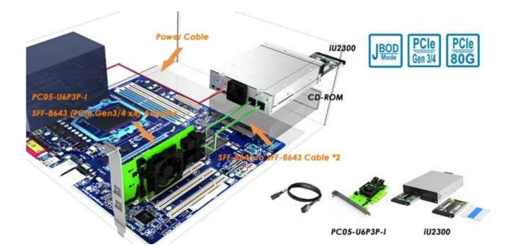
The HBA elevates user storage solutions to new heights with the HiU2300P – a fusion of velocity and inviolability.
