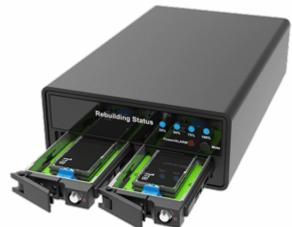
It features a secure, hot-swappable M.2 NVMe SSD tray that enhances airflow to minimize heat buildup, ensuring consistent high-speed performance and extended drive lifespan.
