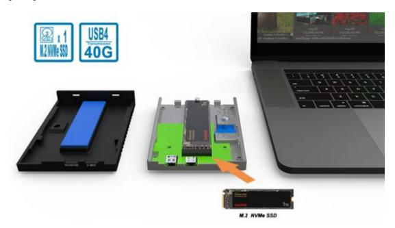
This device, featuring the latest USB 4.0 technology with a 40Gb capacity, is built using M.2 NVMe SSD technology, ensuring transfers up to 40Gb/s. It supports multiple interfaces including USB Type-C and Thunderbolt 3/4.
