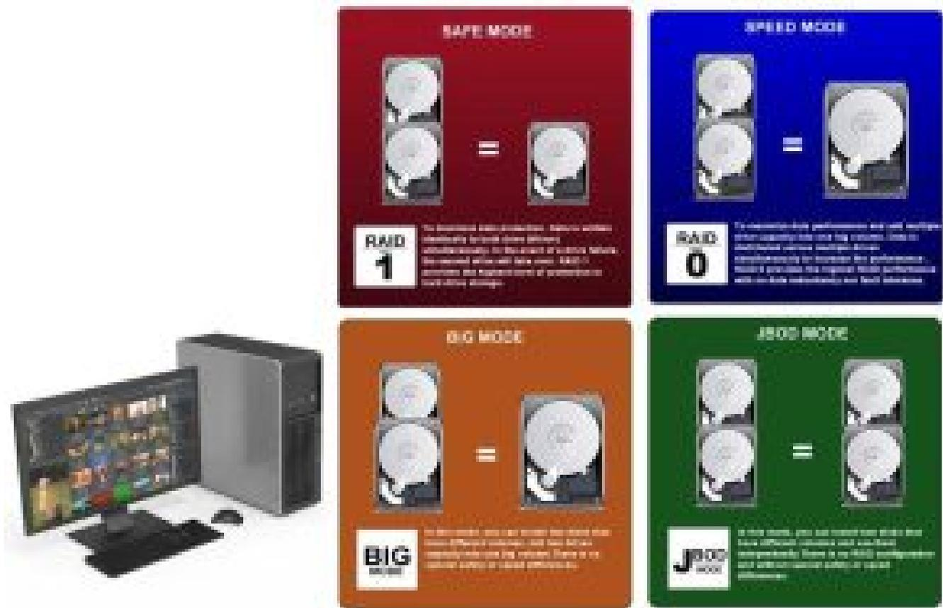
Featuring 4 RAID modes (RAID-1, RAID-0, JBOD, and SPAN (BIG)), the iR2975 enables users to choose the suitable mode based on their specific system needs. For those focused on security and redundancy of their OS, RAID-1 mode with a high-speed SSD hard drive is advisable. On the other hand, if user is seeking enhanced storage performance and capacity expansion, RAID-0 or SPAN mode can be utilized to boost gaming system's performance.
