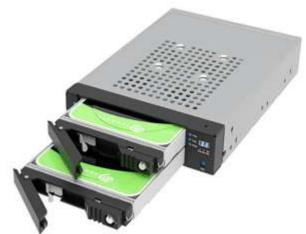
The **iR2977S** elevates traditional RAID-1 storage by combining **real-time redundancy** with **configurable backups** at **1**, **7**, **or 30-day intervals**, ensuring both immediate protection and flexible recovery options.
