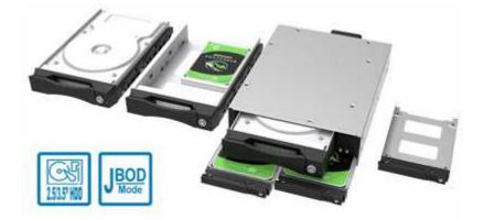
The iT2300 is built in 2-in-1 design, that can be fit in 1x5.25" CD-ROM size and install  $2\times2.5"$  SATA HDD/SSD and  $1\times2.5"/3.5"$  SATA HDD/SSD. It provides JBOD independent capacity mode, so the **3 HDD/SSD data are stored separately**. It also provides the LED indicators on the front panel to make operation and maintenance.
