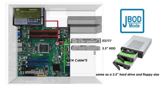
The iT2777 supports 6Gb SATA host interface and SATA 15 pin power supply. It allows  $2 \times 2.5$ " SATA drives to be fitted into  $1 \times 3.5$ " drive space, its size, SATA connector locations and screw holes are the same as 3.5" HDD. It provides JBOD feature and keeps OS and data separately in 2 HDDs/SSDs, so that users could upgrade it with RAID feature from installing a RAID adapter thru SATA cable.
