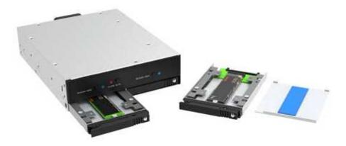
It is capable of supporting 2xM.2 NVMe SSDs of all sizes (2280/2260/2242). The iU2300-U6P3 features high-speed mini SAS (SFF-8643) connector compatible with both PCIe Gen 3 and Gen 4 interfaces and provides versatile application options with its support for JBOD Mode. It also offers compatibility with both U.2 SSD drive and firm's 9.5mm UBOX mini disk tray specifically for M.2 NVMe SSDs.
