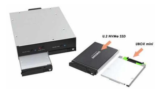
The iU2300-U6P3's disk tray includes an UBOX mini, making it convenient for users to install M.2 NVMe SSDs. If the need arises to use a 2.5-inch U.2 SSD drive, simply remove the UBOX mini after unloading, and then you can install a standard 2.5-inch U.2 SSD drive (with a height of up to 9.5mm).
