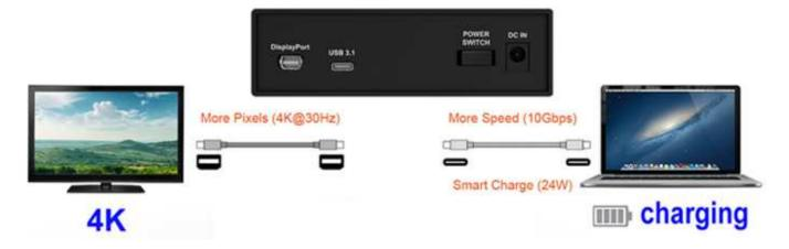
Besides, the 3S2U+ adapter also provides USB PD (Power Delivery) of 24W (12V/2A)/ 18W (9V/2A) / 15W (5V3A) charging for notebook, and 1xDP 1.1a Mini DisplayPort for the  $2^{nd}$  monitor expansion. It is compatible with the existing display port screens, devices that can be connected with DVI, HDMI, and VGA screens.
