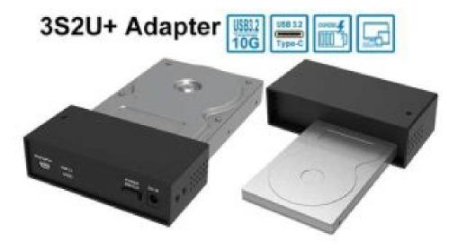
It can install  $1 \times 2.5$ "/3.5" SATA-3 HDD/SSD, provides USB Type C to C cable, and supports drive hot swappable and plug and play.
