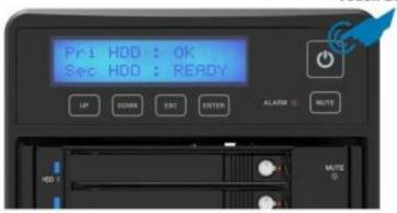
It is designed with the touch setting button and touch power on the front panel. It is more convenience and user friendly for users can touch on/off the power. It also provides visual and audio alarms and mute button. The device will be warning whenever failure occurs, and the buzzer can be turned off to avoid the noise interference.
