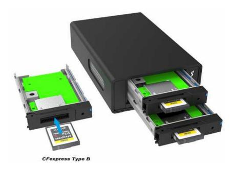
The U2F-B32 is equipped with 2 to install CFexpress adapter and it is built in JBOD mode that can support 2 independent CFexpress Type B storage capacities. The data can be stored separately, just like 2 independent databases. Users could editing photos or videos, transfer data among different storage devices, or back up the import data offsite to meet the various needs in the different computer environments.
