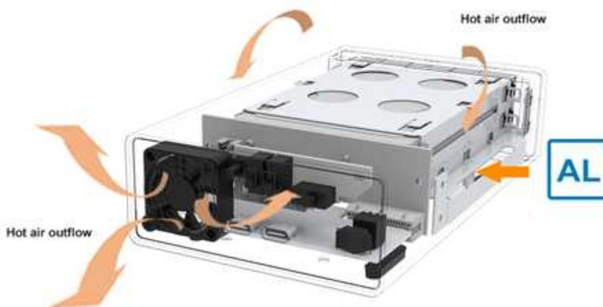
UR2-B32 is made by the durable aluminum housing and designed with the 3cm silent fan that help for heat dissipation with the long time use.
