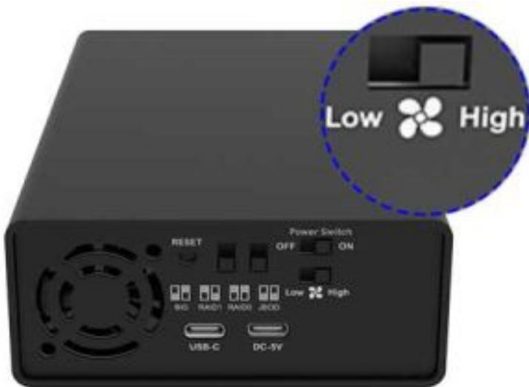
The UR2-B32 have the manual fan adjustment that users can adjust the fan speed to high speed or low speed. User does not need to worry about the fan sound to disturb the work environment, and the device can be still working efficiency.
